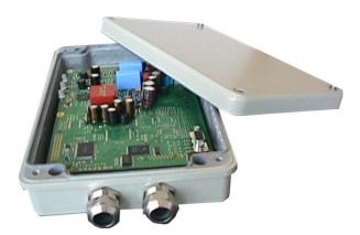
For harsh environments and outdoor use FlexDSL Orion 2 Repeaters are also available in cost effective and high profile aluminum enclosures, extending single or dual pair SHDSL (TC-PAM16/32). It offers Ethernet add/drop functionality (10/100BT, Bridge) and is protected by an IP-67 aluminum housing. The repeater can be powered locally or remotely over the DSL line. Therefore, it is configurable as power "end-point" or "pass-through".
