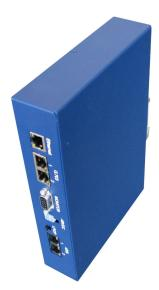
When Rail mounting is a requirement the FlexDSL Orion 2 Repeater with DIN Rail case is the right choice, extending single pair SHDSL (TC-PAM16/32) up to 5.7Mbps. it offers Ethernet add/drop functionality (10/100BT, Bridge) and comes in a blue (RAL 5003) powder coated metal housing with white labeling.
