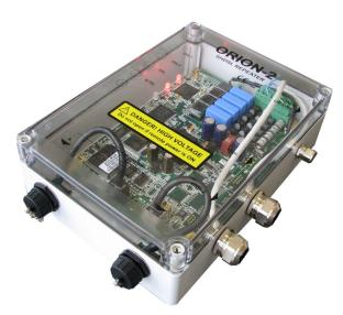
This FlexDSL Orion 2 Repeater extends single or dual pair SHDSL (TC-PAM16/32). It offers Ethernet add/drop functionality (10/100BT, Bridge) and is protected by an IP-67 plastic housing. The repeater can be powered locally or remotely over the DSL line. Therefore, it is configurable as power "end-point" or "pass-through".
