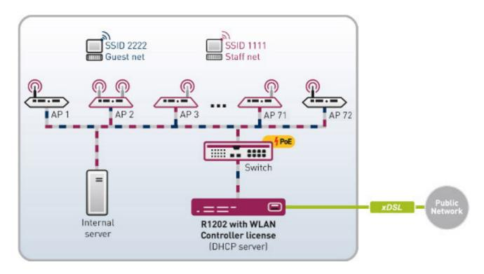
For up to 72 access points, the bintec Rxx02 series (e.g. RS1202) hardware is required. To run it, you require a WLAN controller licence on a bintec router.
