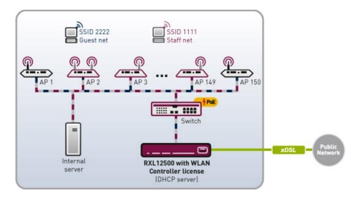
For 150 access points, a bintec RXL series hardware is required. To run it, you require a WLAN controller licence on RXL series.
