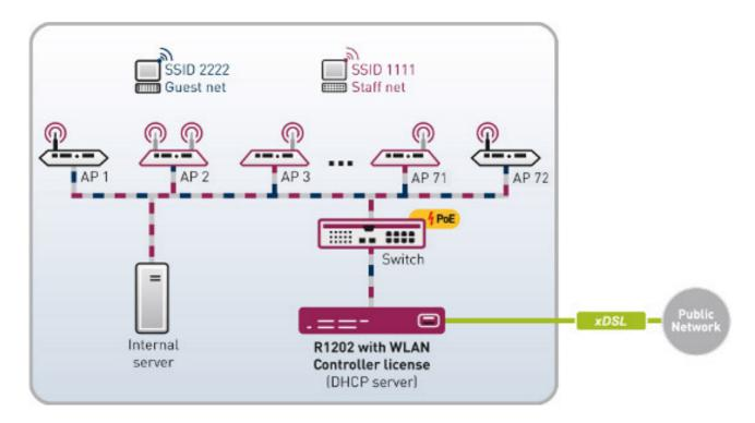
For up to 12 access points, the bintec RS series (RS123, RS353xx) hardware is required. To run it, you require a WLAN controller licence on a bintec router.
